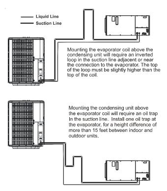
Insulation is necessary to prevent condensation from forming and dropping from the suction line. Armflex (or satisfactory equivalent) with 3/8" min. wall thickness is recommended. In severe conditions (hot, high humidity areas) 1/2" insulation may be required. Insulation must be installed in a manner which protects tubing from damage and contamination.
